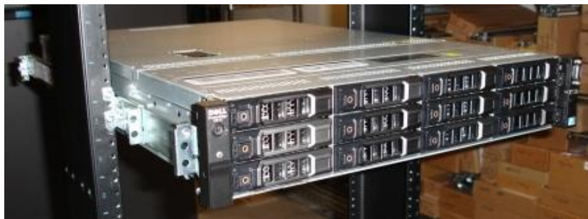
Figure 10. R515 Mounted in the B4 Static Rails in 2-Post Center Mount Configuration
