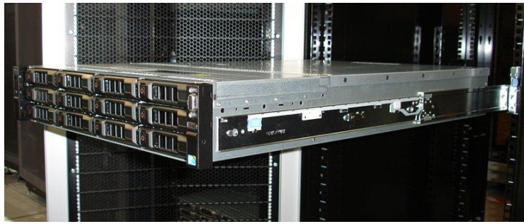
Figure 8. R515 Mounted in B3 Sliding Rails
